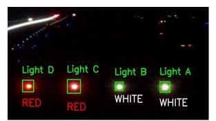
Our solution can be used in commissioning, inspection & calibration of PAPI systems. The operation can be carried out during the day or night, which allows flexible scheduling. Flight checks by aircraft for PAPI can now be fully replaced by our solution, which only takes a few minutes to perform all the measurements. Our inspection method is more precise thanks to custom software, specific procedures, RPAs with precise GNSS & computer vision which automatically detects colour transitions.
