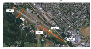
The procedures for measuring NAVAIDs have been designed following ICAO (Doc 8071) and FAA (8200) recommendations. All procedures translate to meaningful and relevant measurements that are used in ground checks, commissioning and flight inspections.
