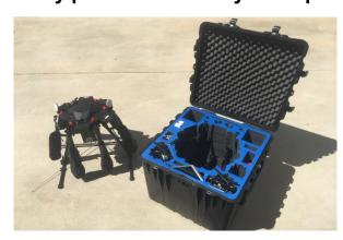
The complete system, including the drone, fits in a 75x75x75 cm rugged transport case. The case can be shipped with any courier or carried as special checked-in baggage with most airlines.
