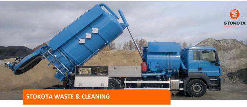
Stokota produces industrial cleaning vehicles and vacuum trucks for hazardous products, wet and dry materials and sewage cleaners since 1992. Supersuckers, high-pressure units or combi-units on rigid and semi-trailer chassis with vacuum tank, water tanks, jetting pumps and numerous options are available. All units can be made according ADR and with SIR approval.
