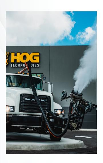
Water blasting works by directing pressurized streams of water at a surface to accomplish a given task. The needlesharp water jets of a properly designed water blasting system will reach like tiny fingers into the pores or grooves of the asphalt or concrete with unmatched effectiveness.
