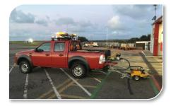
Using a Findlay Irvine MK2 Grip Tester the 100m section was recorded at **0.93**, compared to pre-application grip level of **0.83**
